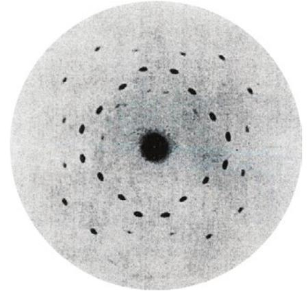
Max von Laue discovered that X-rays beamed through a crystal onto a photographic plate acquire a clear diffraction pattern.
