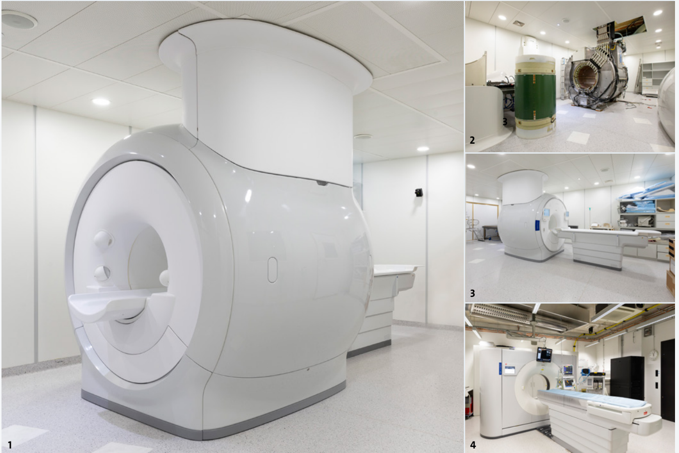
1: The new Philips MRI gantry; in white with light and breath camera / 2: Exposed magnet, with next to it the new gradient coil to be installed in the magnet / 3: The new Philips MRI gantry with examination table; new in white and blue / 4: The new Philips IQon Spectral CT
