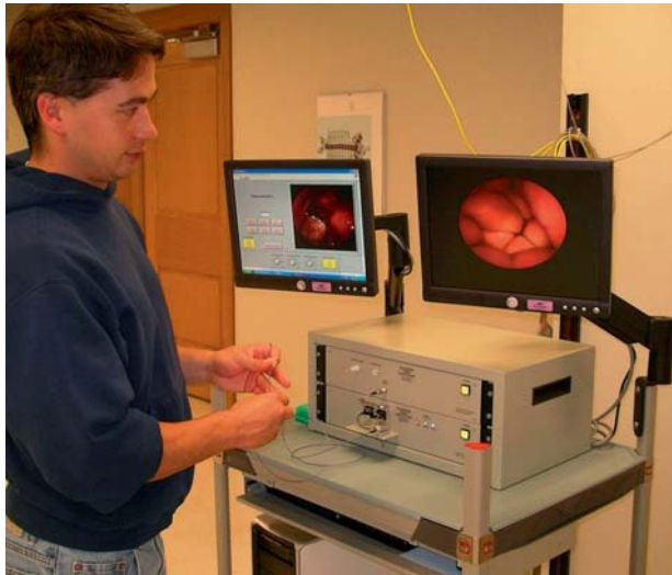
Figure 5 (online color at: www.biophotonics-journal.org ) Photograph of SFE system being used to image within a closed fist of the operator.
