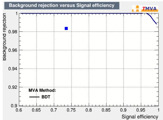
Figure 4.40: Curve: the ROC curve from the BDT method. Blue dot: the result from the cut-based method.
