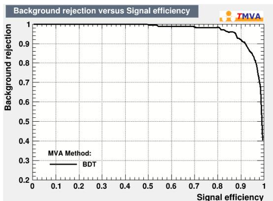
Figure 4.12: The ROC curve of BDT method.
