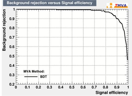
Figure 4.14: The ROC curve of BDT method.
