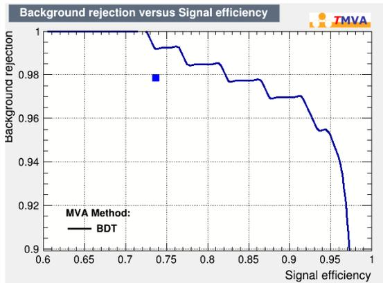
Figure 4.37: Curve: the ROC curve from the BDT method. Blue dot: the result from the cut-based method.
