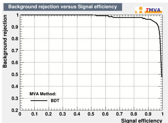
Figure 4.9: The ROC curve of BDT method.
