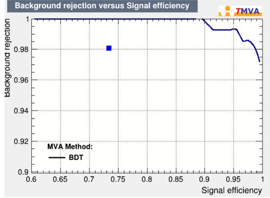
Figure 4.39: Curve: the ROC curve from the BDT method. Blue dot: the result from the cut-based method.
