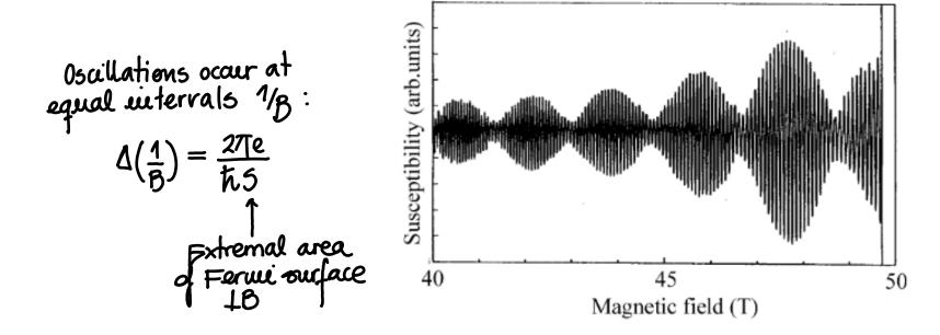
Figure 9.9: de Haas-van Alphen oscillations in Pt at 4.2 K with B parallel to [111]. The data have been recorded using a pulsed magnetic field. Note the presence of two frequencies of oscillations due to two extremal orbits about the Fermi surface. The y axis, labelled "susceptibility", represents the voltage V induced in the coil divided by (dB/dt), leaving a quantity proportional to the differential susceptibility (dM/dB) (Data from S. Askenazy, Physica B 201, 26 (1994).)
