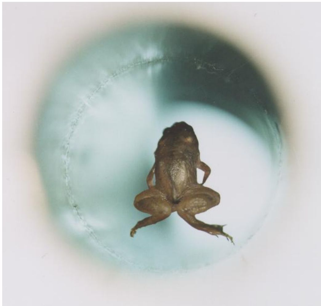
A live frog levitates inside a 32 mm diameter vertical bore of a Bitter solenoid in a magnetic field of about 16 T at the Nijmegen High Field Magnet Laboratory.
