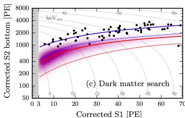
We derived the most stringent limits on the WIMP-nucleon cross section for WIMP masses above 10 GeV/c<sup>2</sup>, with a minimum at 7.7x10<sup>-47</sup> cm<sup>2</sup>.
