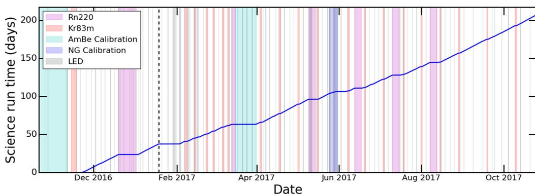
Our Data Acquisition system collects science data with 99% efficiency. Since late 2016, we have accumulated 34.2 (Run 0) and ~200 (Run 1) live days of data.
