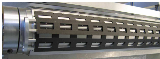
Segment of the CMS pixel detector support structure.
