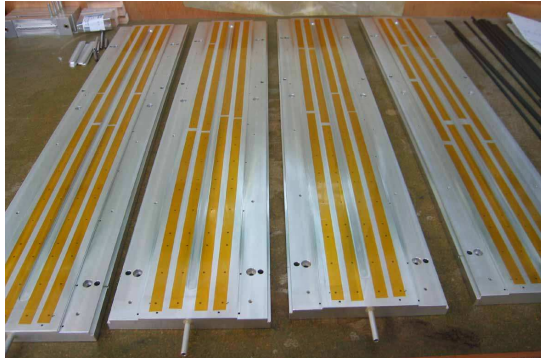
Cooling plates for the LHCb detectors.
