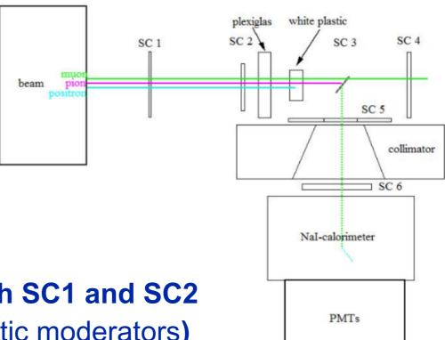
Beam particles pass through SC1 and SC2 (and are slowed down in plastic moderators)
