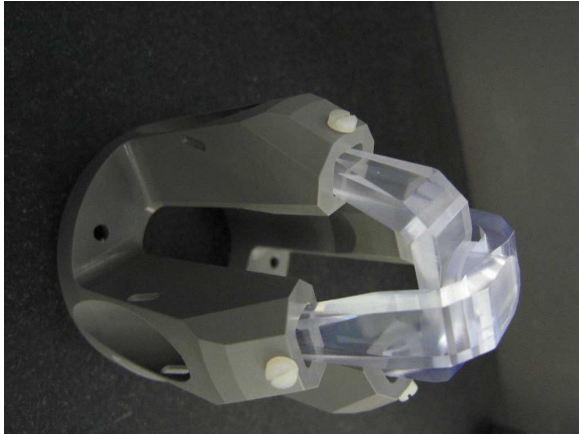
Figure 5.5: The four-plane wedged degrader used in 2008 to measure the pion trajectory before wrapping. The beam enters from the left.
