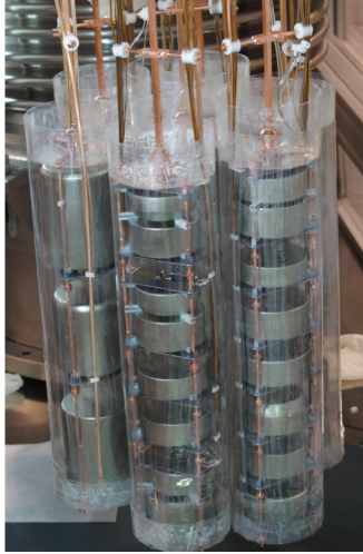
Figure 4: Full assembled Phase II array with nylon mini-shrouds. The figure is taken from [24].
