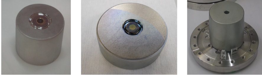
Figure 6: Photos of a coaxial (left), BEGe (centre) and IC (right) detector. The photos are taken from [20].
