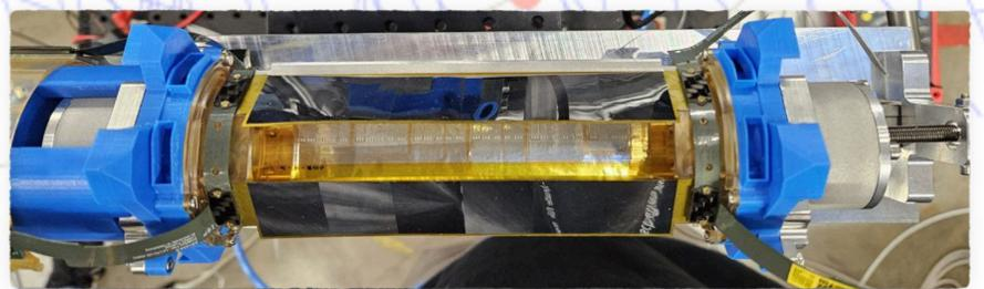
Two ladders setup in latest test beam at PSI
