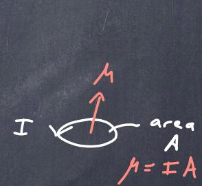
This is the magnetic moment of a charge particle depends on angular momentum, charge, & its mass.
