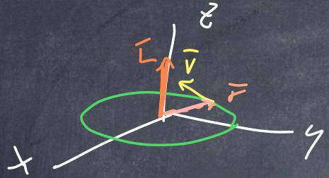
A particle moving in a circle in the  $x-y$  plane with a velocity  $\vec{v}$ , its speed  $|\vec{v}|$  is constant.
