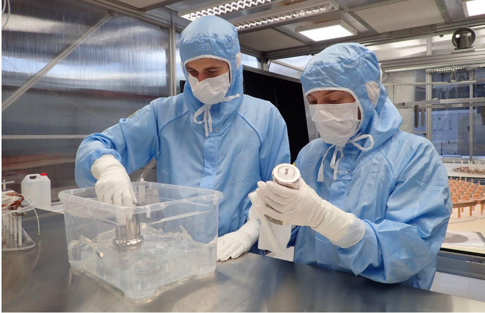
Figure 6.15: PMTs being cleaned by dipping in an ethanol bath and wiping.
