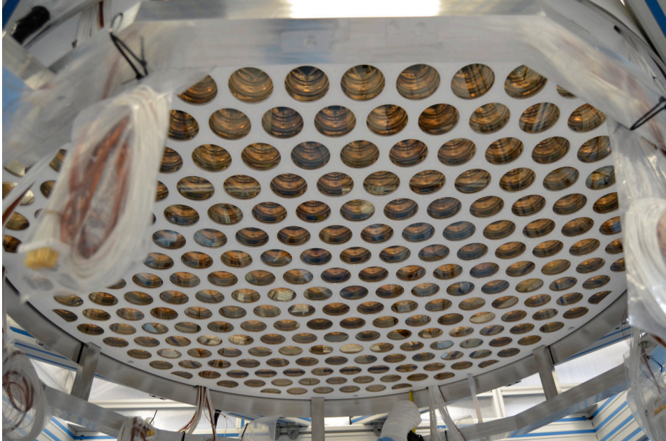
Figure 6.14: The top PMT array, hanging in the bell before the field cage was added.
