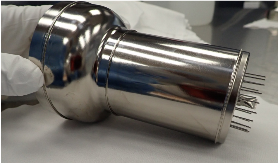
Figure 6.16: Deposits on a PMT after cleaning and drying. These were found to be released from cleanroom gloves when in contact with ethanol, and easily removed by wiping the PMT once more.
