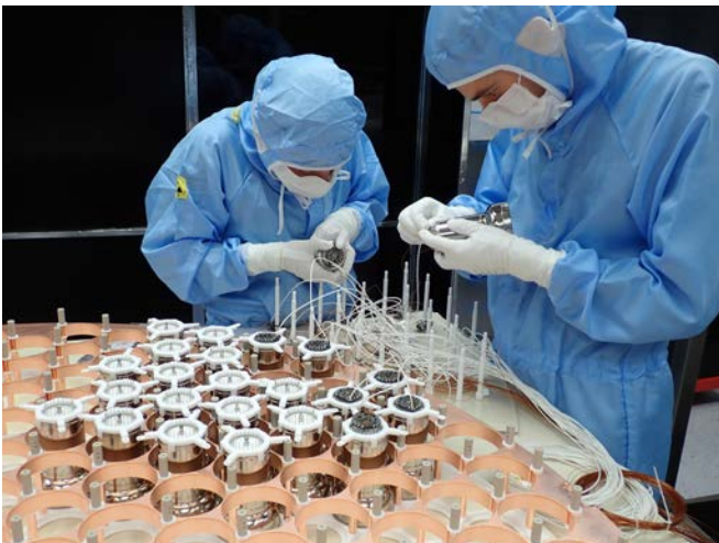
Figure 4.17: Picture during the PMT array assembly in above ground cleanroom at LNGS. The PMTs were placed in the array following the cabling plan, after installing the corresponding base.
