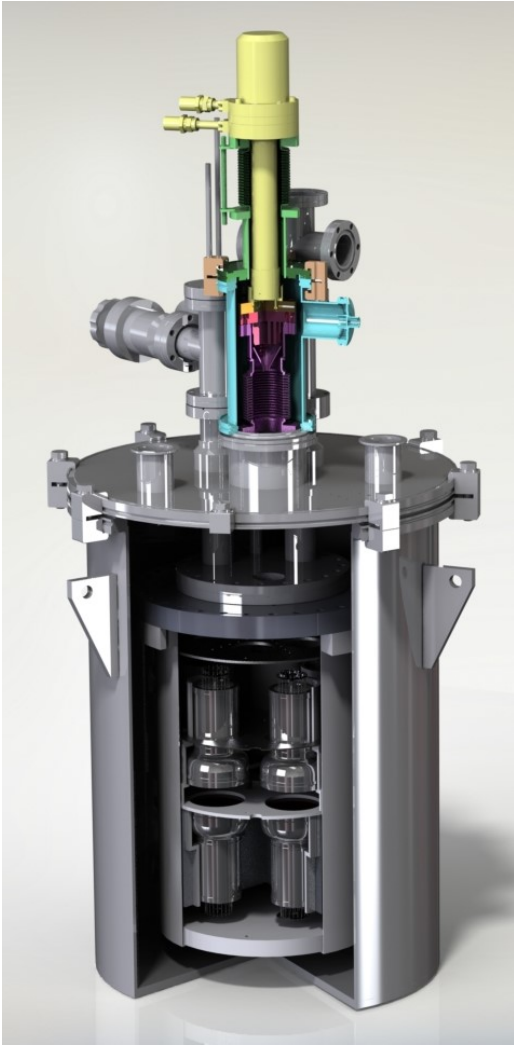
Figure 4.6: Render of the MarmotX testing facility. The PMTs are hosted in a two-array structure inside the inner cryostat and inserted inside the outer cryostat. The region among the two cryostats is evacuated to ensure good thermal insulation. The xenon is liquefied at the top by the PTR. Several ports allow the cable connection from the air to the xenon side to perform the PMT testing. Figure by J. Franchi.
