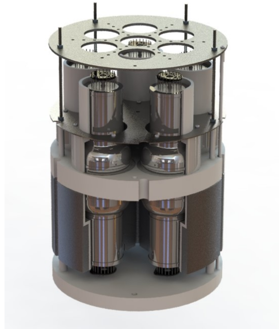
Figure 4.7: Render of the PMT support structure used in the MarmotX testing facility. The two-sided structure of PMT arrays can be appreciated. Figure by J. Franchi.
