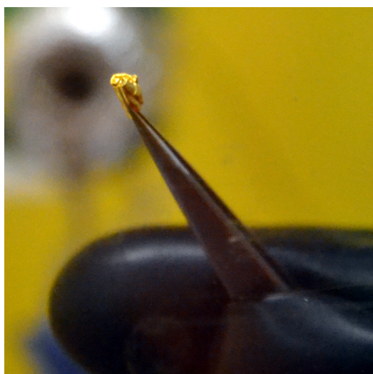
(e) Folding of the inner gold foil, containing the \text{ThO}_2 .
