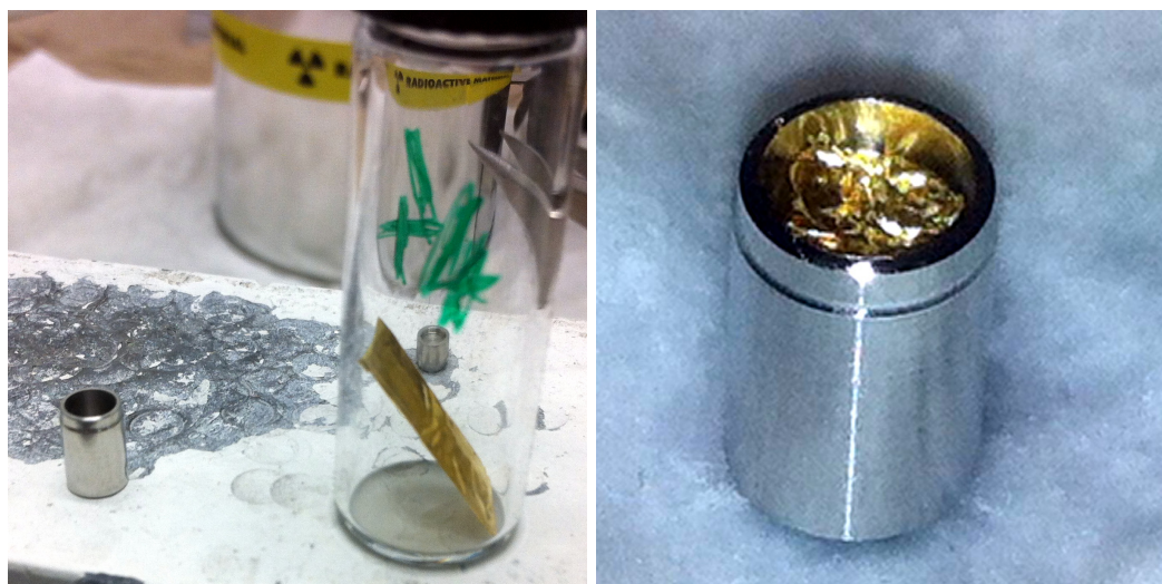
(a) Inner source capsule (left) with the ^{228}\text{Th} in the gold envelope (right). (b) Gold envelope pressed in the inner capsule.
