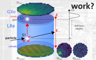
XENONnT is a dual-phase time projection chamber: filled with liquid xenon and a thin gas layer at the top. An energy deposition from a particle produces a prompt light (S1) and a delayed charge (S2) signal. These are measured with photomultiplier tubes. From S1 and S2 we reconstruct the position, energy and type of the interaction.
