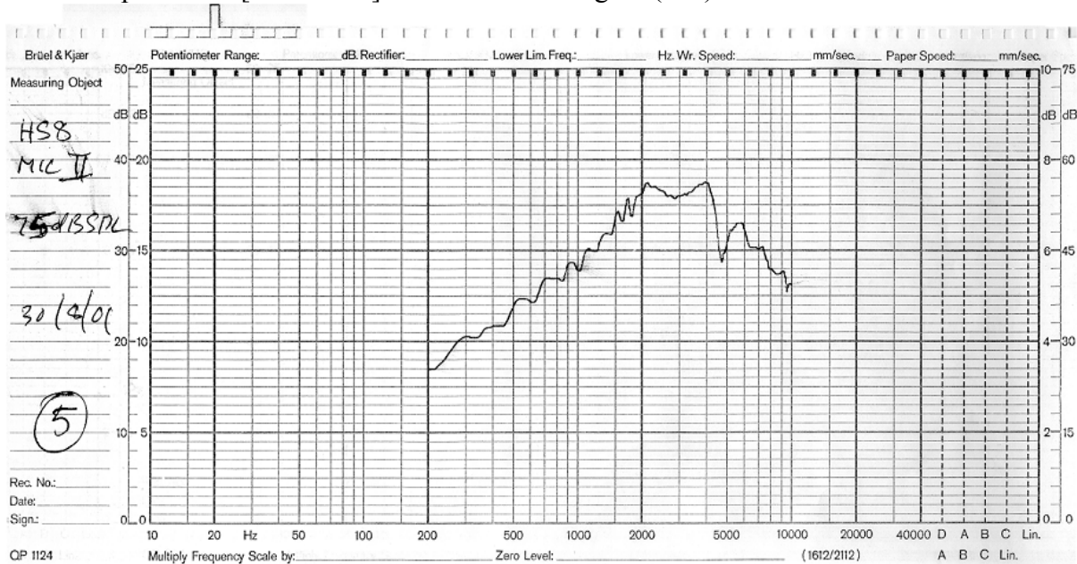
Figure (D.5): Microphone transfer function according to Cochlear documents.
